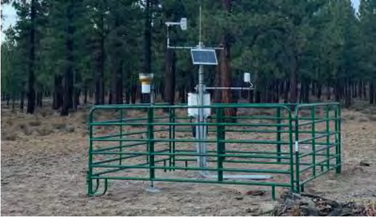
Figure 4. Station with Round pen used for an exclusion. Surface Meteorology and soil moisture and temperature.
